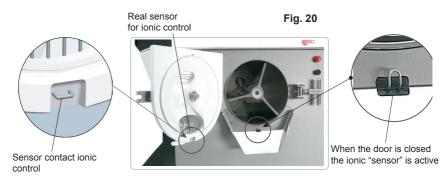
In addition to all this, the ionic system exploits the potential of a new electronic device whose use in ice-cream machines has been patented by BRAVO:
